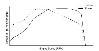
Get the right power curve for your needs. Mack's Maxidyne<sup>®</sup> engine rating has extended RPM ranges and high torque rise for off-road and jobsite use. MaxiCruise<sup>®</sup> offers both power and economy for off-road and on-highway.
