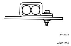
Fig. 29 Provide Proper Clamp Support
