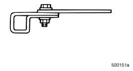
Fig. 28 Avoid Installation Where Fastener is Perpendicular to Ground
