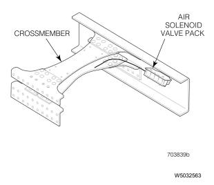
Fig. 1 Air Solenoid Valve Pack Location
