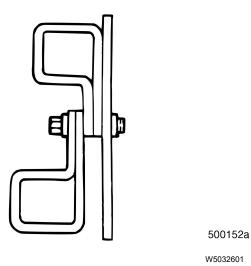
Fig. 30 Installing Two Clamps on One Fastener
