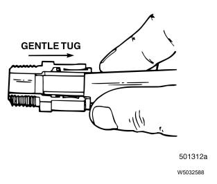
Fig. 17 Ensure Tubing is Secure
