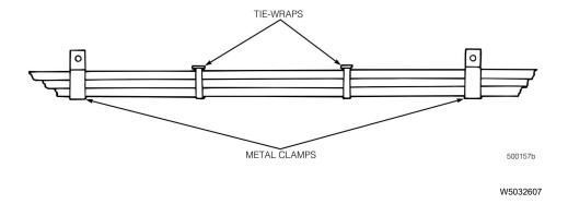
Fig. 35 Metal Clamps for Primary Support, Tie Wraps for Bundling
