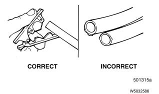
Fig. 15 Use a Tubing Cutter for Proper Cut Edges
