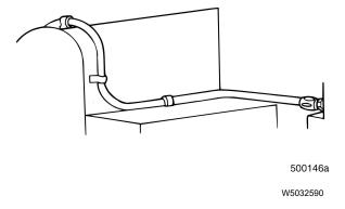
Fig. 19 Flexible Air Line Following Contour of Equipment
