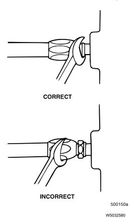
Fig. 10 Tightening Male-End Fittings
