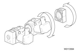
Fig. 2 Assembling Solenoid Valve
