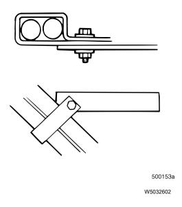
Fig. 31 Avoid Inadequate Clamp Support
