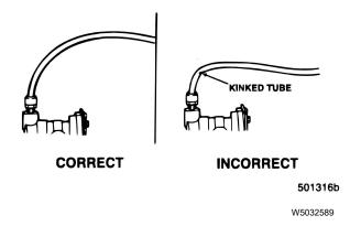
Fig. 18 Inspect Final Installation
