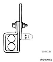
Fig. 32 Proper Backing for Multiple-Hose Clamp Installations
