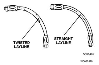
Fig. 9 Twisted and Straight Laylines
