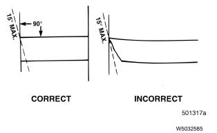
Fig. 14 Clean, Square Cut Tubing Edge
