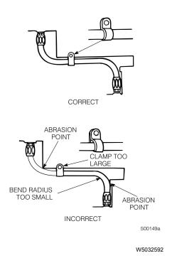
Fig. 21 Route and Clamp Line to Prevent Abrasion
