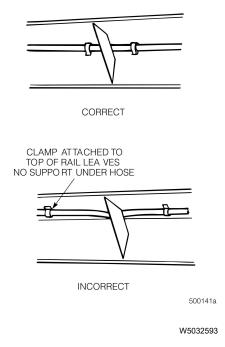
Fig. 22 Route and clamp to avoid sharp edges
