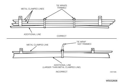
Fig. 36 Use Tie Wraps for Primary Support of Additional Hose(s)
