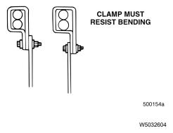
Fig. 33 Inverted Clamp Installation
