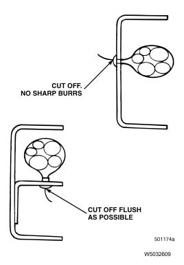
Fig. 37 Installing Button-Head Tie Wraps
