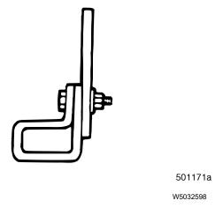
Fig. 27 Preferred Clamp Installation
