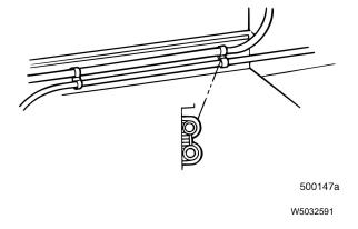
Fig. 20 Air Line Pairs Routed Parallel
