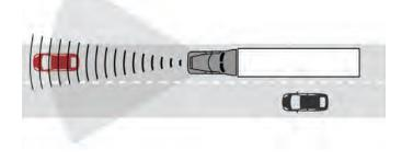
When Bendix Wingman Fusion can definitively identify the large, stationary object as a vehicle, the system will alert the driver with 3.5 seconds notice. Then, if necessary, it will automatically apply the brakes.
