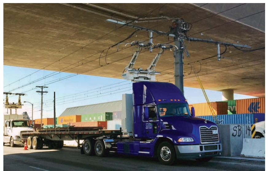
A prototype Mack® Pinnacle™ axle back model equipped with a proprietary plug-in hybrid electric driveline recently participated in a zero-emission eHighway demonstration in Carson, California. The demo was conducted as part of a project with Siemens and sponsored by the South Coast Air Quality Management District.
