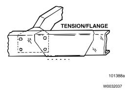
Fig. 27 Acceptable Reinforcement Plate Location
