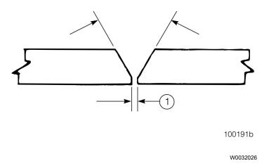
Fig. 16 Aligning Joints for Welding
