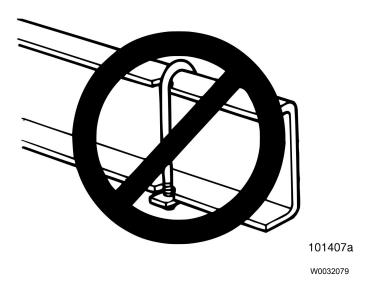
Fig. 11 Do Not Notch Frame Rail Flange
