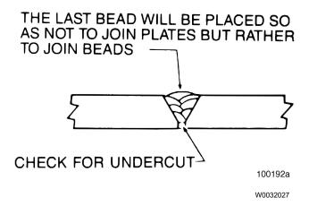
Fig. 17 Proper Weld
