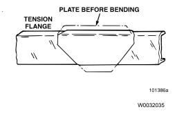
Fig. 25 Acceptable Reinforcement Plate Design
