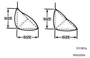
Fig. 19 Acceptable Fillet Weld Profile
