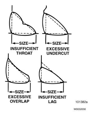
Fig. 20 Unacceptable Fillet Weld Profiles
