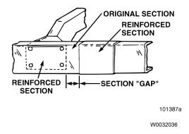
Fig. 26 Unacceptable Reinforcement Plate Location
