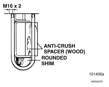
Fig. 10 U-Bolt with Rounded Shim and Anti-Crush Spacer
