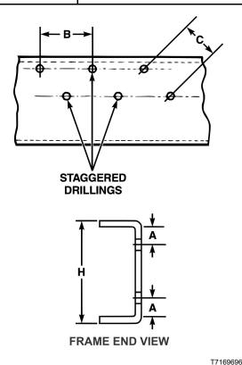
Fig. 33 Drilling Locations in Frame Webs
