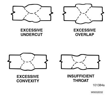
Fig. 22 Unacceptable Butt Weld Profiles
