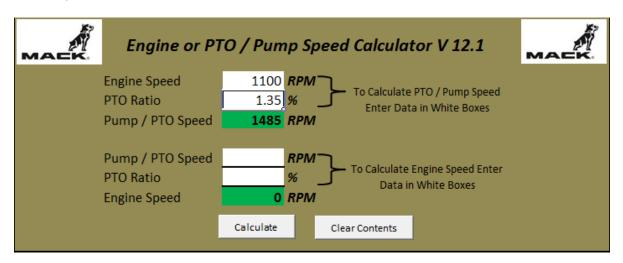
3. Go back to the Pump Info worksheet to see what flow rate we can expect from the F1-101 pump with 1485 RPM. Using the calculator to the right of the pump table, select F1-101 from the dropdown list and enter 1485 RPM. Click Calculate and the GPM that this offers is 40.1 GPM. But the body builder advised that we don't exceed 40 GPM and the RPM is still higher that requested.
