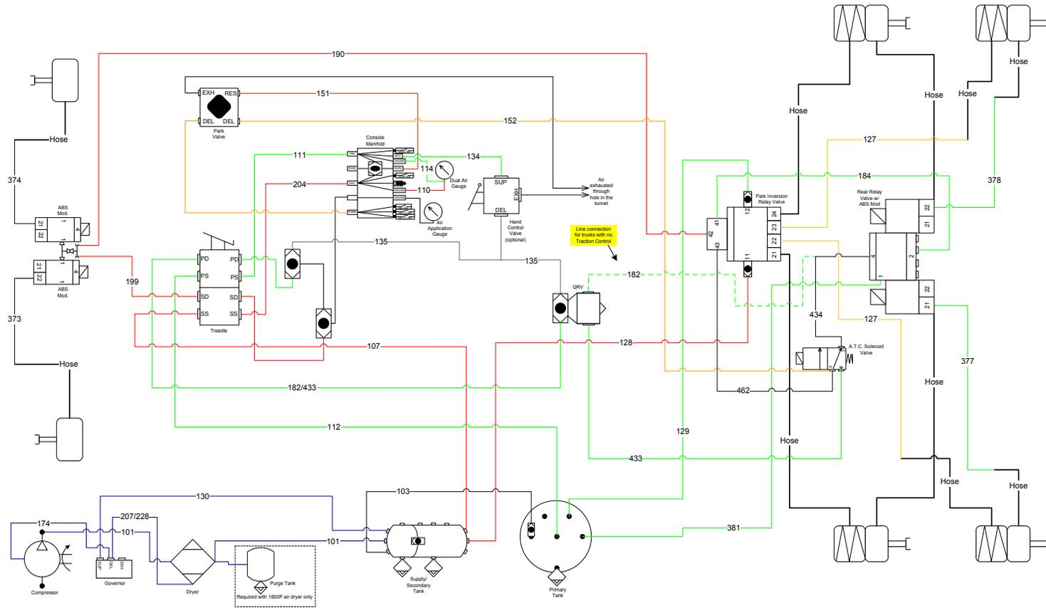
\* Assume a Bendix front axle modulator arrangement for this page, and subsequent pages
